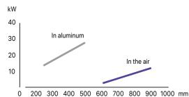
The power ratings range from 2 to 12kW in the air and from 14 to 27kW in aluminum at 700°C, corresponding to heating lengths from 250mm to 900mm.
